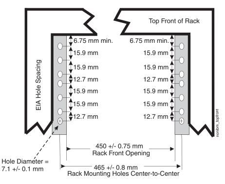
Figure 92. Rack specifications dimensions, top front view
